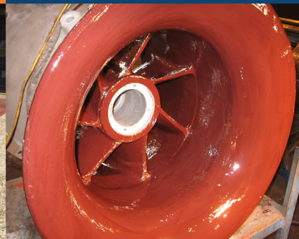
VERTICAL PUMP RESTORED
