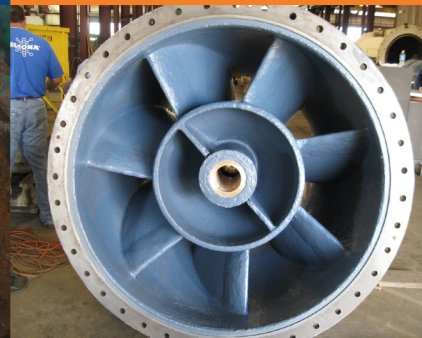
CENTRIFUGAL PUMP RESTORED
