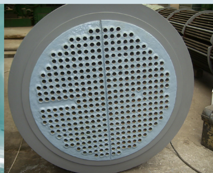
HEAT EXCHANGER RENEWED
