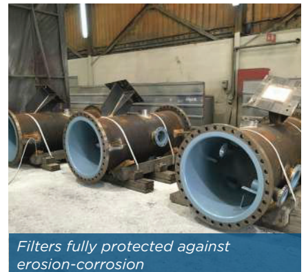
Tank coated with Belzona 5811
