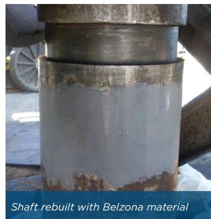
Keyway housing and shaft repaired with Belzona material
