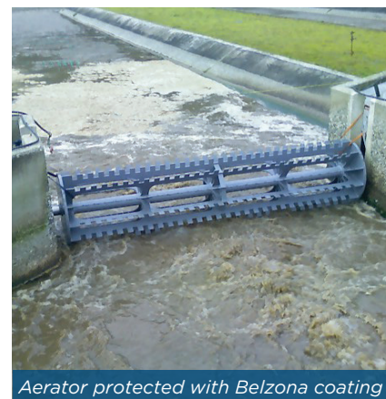
Rebuilt and protected against abrasion
