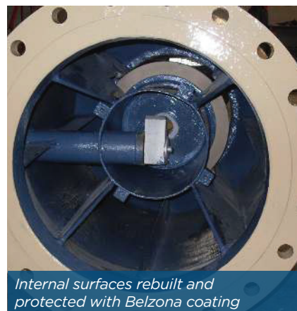
Pump internals coated with Belzona materials for long-term corrosion protection
