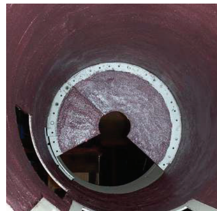
Rebuilt and protected against abrasion
