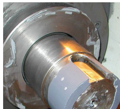
Keyway housing and shaft repaired with Belzona material
