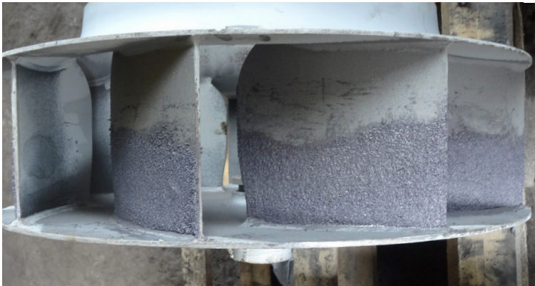
Belzona 1812 (Ceramic Carbide FP) Ceramic-filled high abrasion and wear-resistant epoxy repair composite, particularly suitable for fine particle abrasion.
