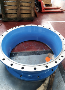
Belzona 1311 (Ceramic R-Metal) Ceramic-filled erosion-corrosion-resistant epoxy metal repair composite.
