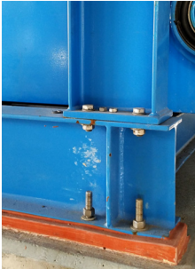
Belzona 7111 Pourable chocking/grouting material designed to spread evenly across uneven surfaces to endure physical and thermal shock.
