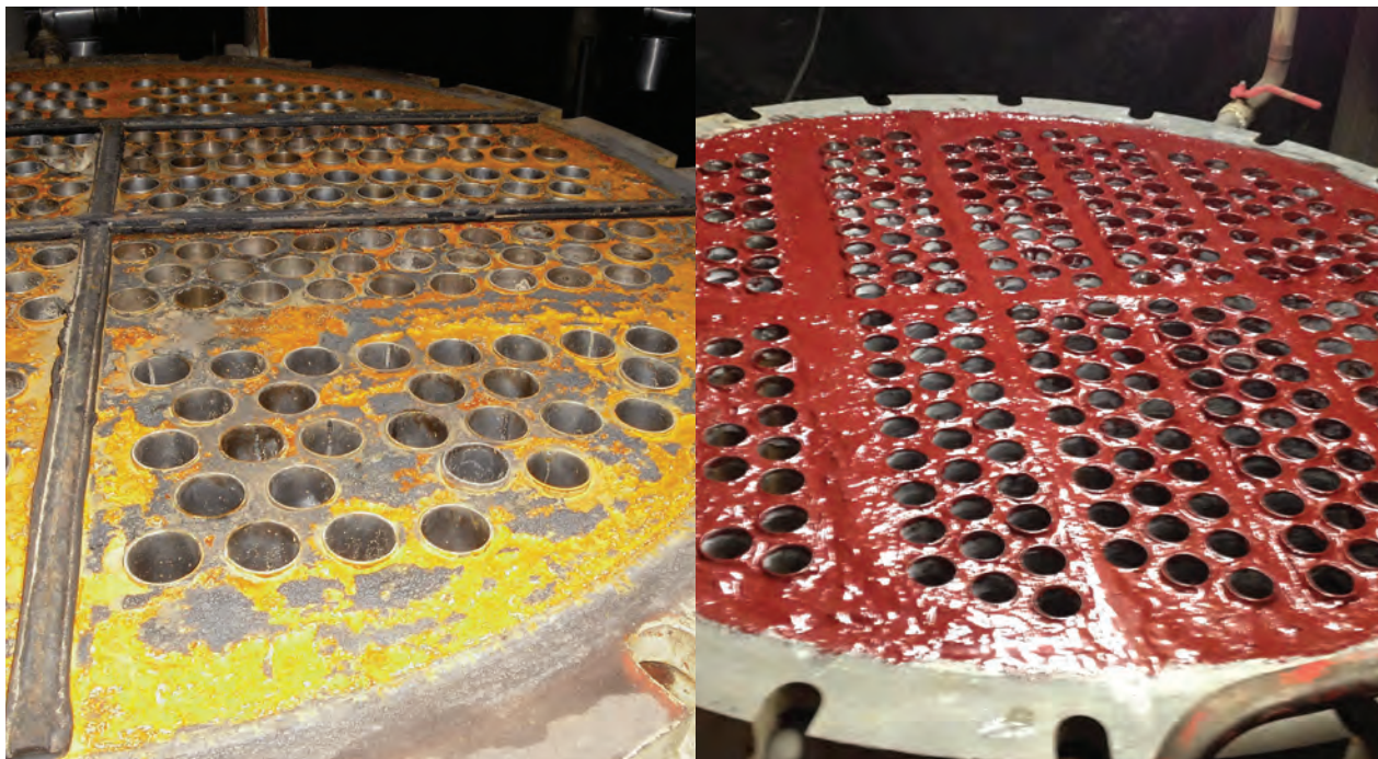
Degradation of surface due to high temperature acidic media
