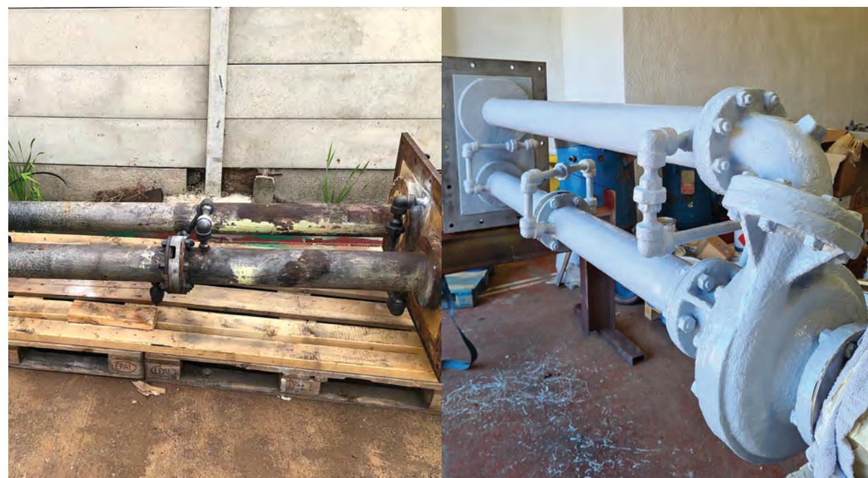
Short working life of pumps due to high corrosion
