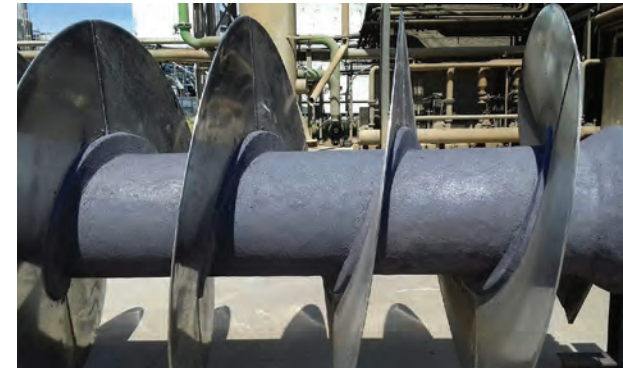
Abrasion resistant coating extends service life
