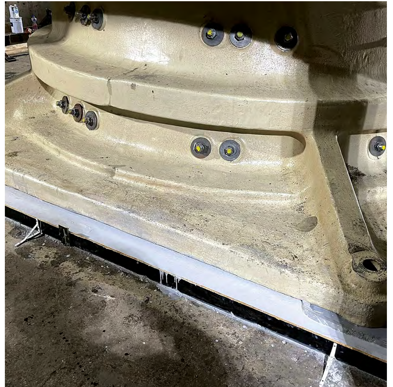
A crusher base stabilized using Belzona anchoring solutions
