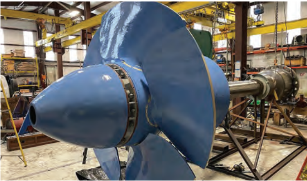
Kaplan turbine rebuilt and protected
