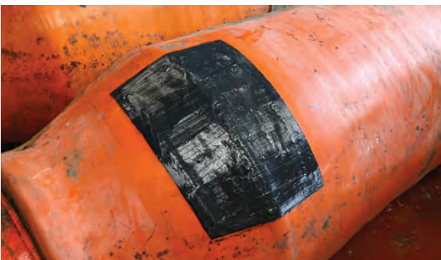
Rubber covers on fuel hoses repaired
