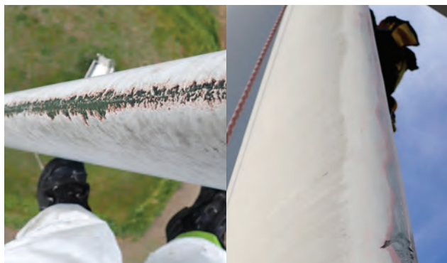
Rain erosion repaired with Belzona leading edge protection solutions
