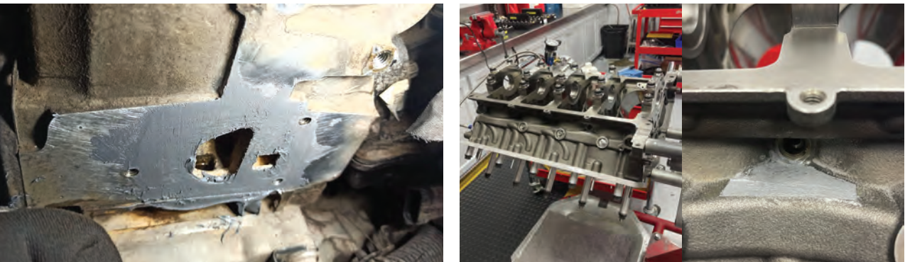
Engine block leaking coolant repaired Damaged engine case repaired with Belzona
