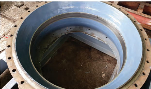
Valve repaired and protected from sea water erosion
