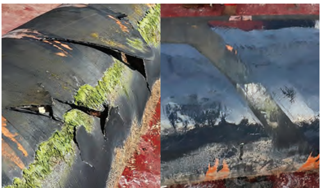
Repaired floating hose damaged by collision with a ship's propeller
