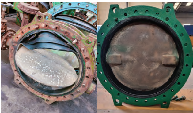
Butterfly valve rubber repaired
