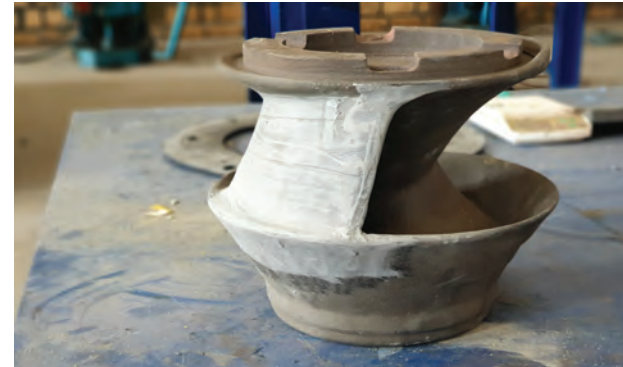
Eroded pump impeller repaired and protected
