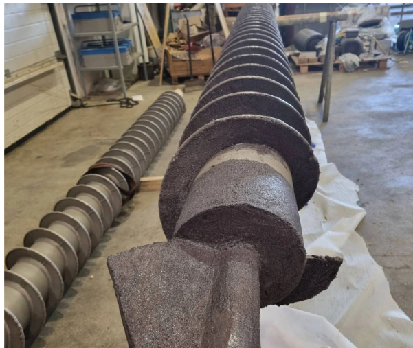
Screw conveyor from the cement industry protected with Belzona.
