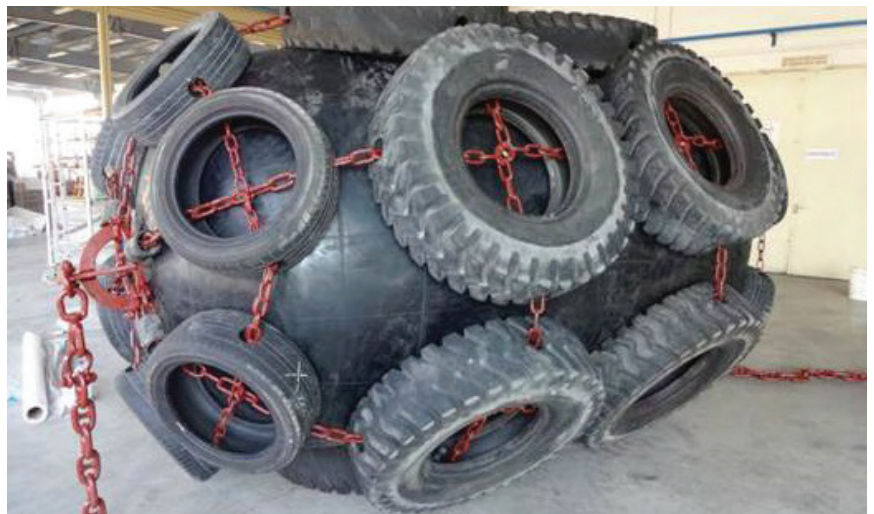
Yokohama fender repaired with Belzona
