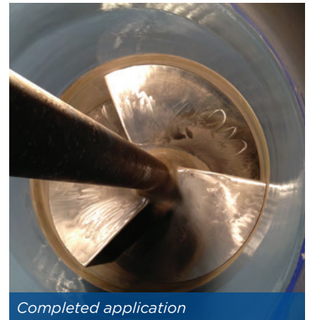
Propeller areas rebuilt and protected
